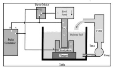
Fig.1: Working principle of EDM[8]
